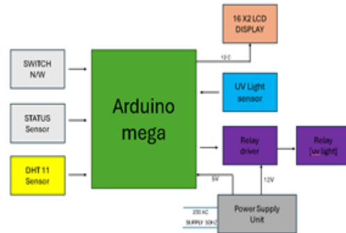
Fig1: Circuit Design of Dip Coating
