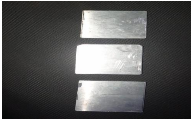
FML samples for corrosion test
