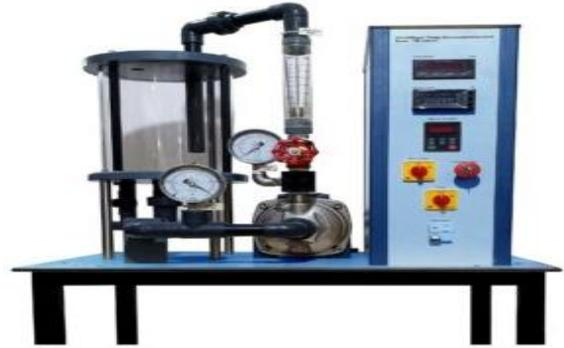
Fig. 1. Experimental set-up of impact of jet.
