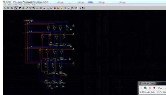
Fig 5.3: Schematic designing of 4 x 4 Braun multiplier
