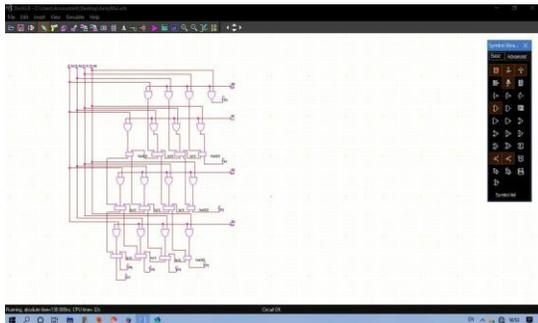
Fig 1.1 : Schematic Design of 4 x 4 Array Multiplier
