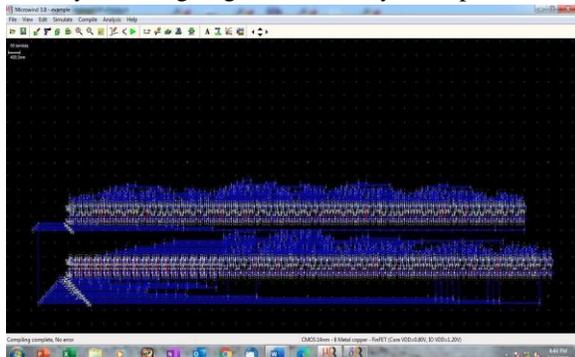
Fig 5.2: Layout designing of 4 x 4 Array multiplier
