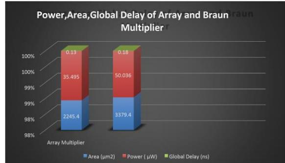
Fig 7.1: Power, Area, Global Delay comparison of Array and Braun Multiplier.
