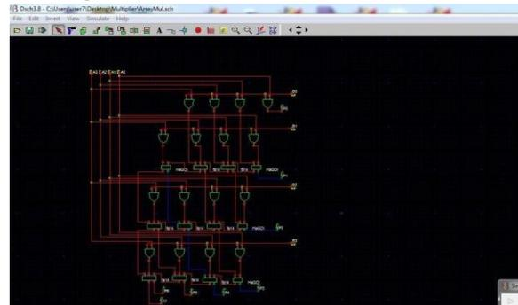
Fig 6.1.1: Simulation of 4 x 4 Array multiplier
