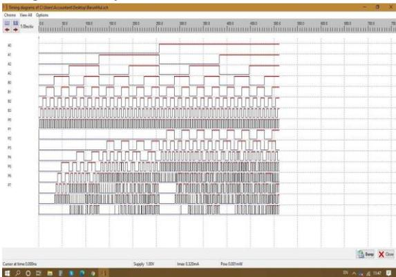
Fig 6.2.2 : Waveform of 4 x 4 Braun Multiplier.
