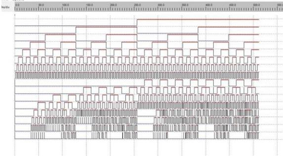
Fig 6.2.1: Waveform of 4 x 4 Array Multiplier.
