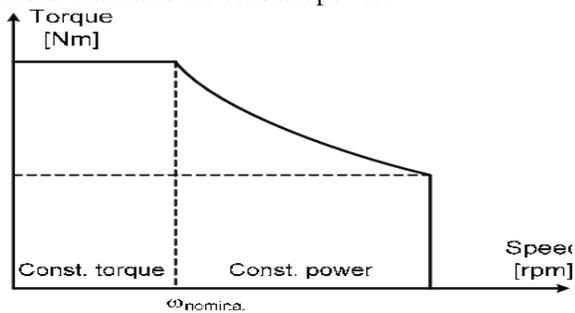
Fig.6. Ideal torque characteristics of PMSM
