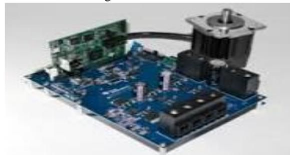
Fig.4. PMSM Motor and Motor Driver
