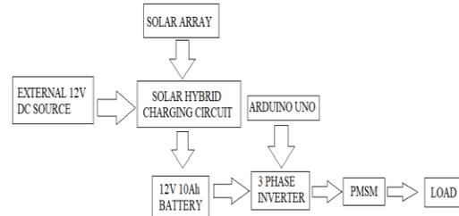
Fig.7. Block diagram of Solar fed PMSM drive using Arduino
