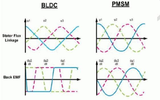
Fig.5. PMSM vs BLDC Waveforms
