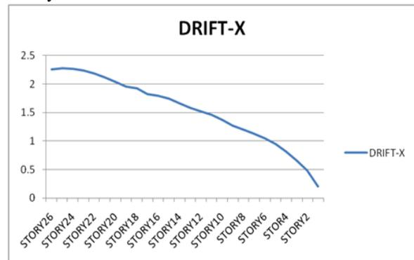
Fig.7: Maximum Drift of structure
