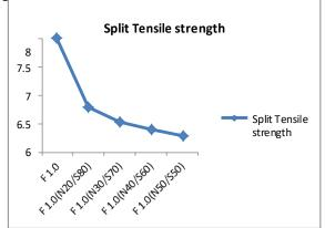
Fig -3: Split Tensile Strength of SCC In split tensile strength, the strength gets influenced by dosage of fibers for reinforcement. The mix id F 1.0 (N80/S20) is found optimum under the category of split tensile strength.
