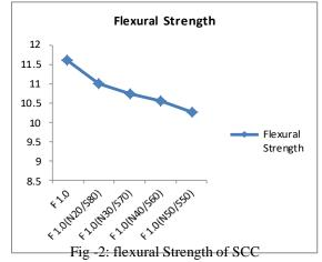
The mix id under the category of Flexural strength F 1.0 (N20/S80) can be chosen optimum.
