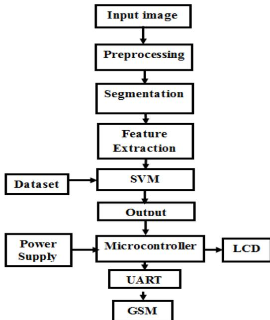
Fig 4.2 Testing Section
