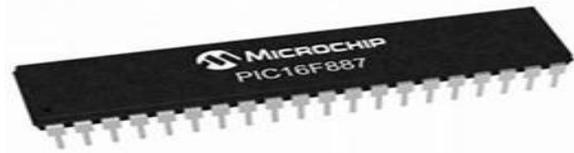
The PIC16F887 is an 8-bit microcontroller from microchip. The IC also has 2 comparators, 2 timers and supports SPI, I2C and UART communication protocols. It can operate at a speed up to 20MHz with external oscillator and also has precision internal oscillator tunable between 8MHz to 32KHz
