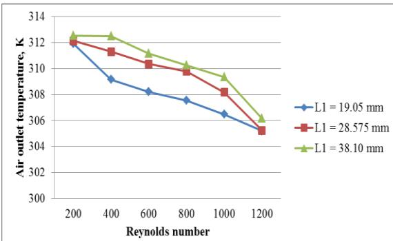
Fig. 4: Effect of varying longitudinal tube pitch on air outlet temperature variation for Wavy fin In-line Configuration
