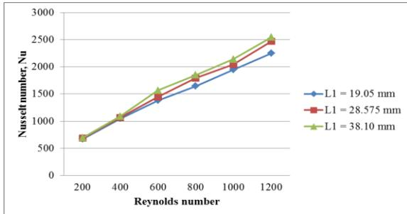
Fig. 26: Effect of varying longitudinal tube pitch on Nusselt number variation for wavy fin staggered configuration
