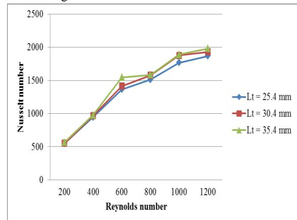
Fig. 13: Effect of varying transverse tube pitch on Nusselt number variation for Wavy fin In-line Configuration
