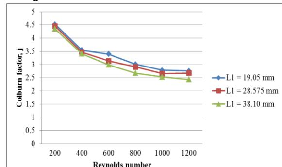
Fig. 28: Effect of varying longitudinal tube pitch on Colburn factor variation for wavy fin staggered configuration
