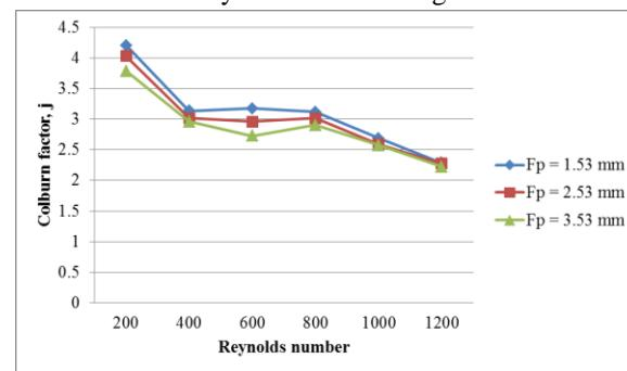
Fig. 21: Effect of varying fin pitch on Colburn factor variation for Wavy fin In-line Configuration
