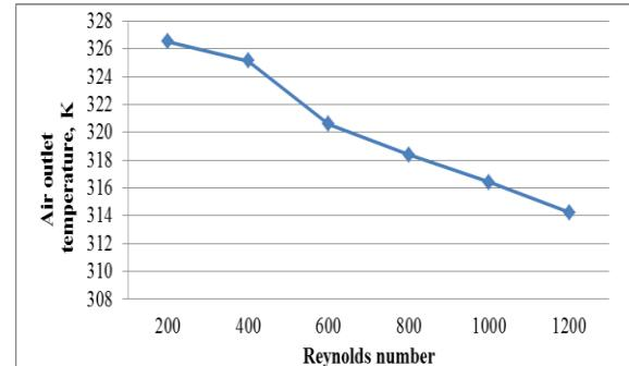
Fig. 22: Air outlet temperature variation for wavy fin staggered configuration
