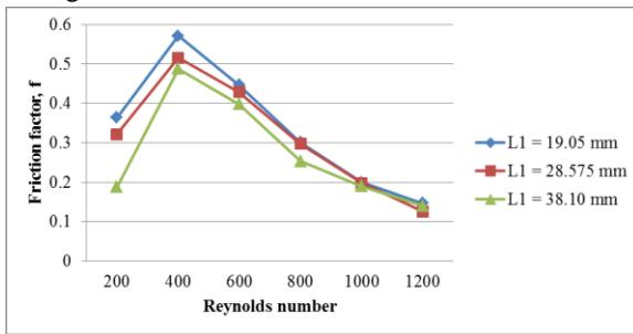
Fig. 27: Effect of varying longitudinal tube pitch on friction factor variation
