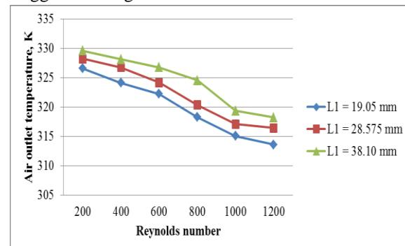
Fig. 23: Effect of varying longitudinal tube pitch on air outlet temperature variation for wavy fin staggered configuration
