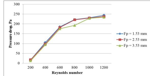
Fig. 36: Effect of varying fin tube pitch on pressure drop variation for wavy fin staggered configuration
