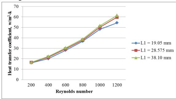
Fig. 25: Effect of varying longitudinal tube pitch on heat transfer coefficient variation for wavy fin staggered configuration
