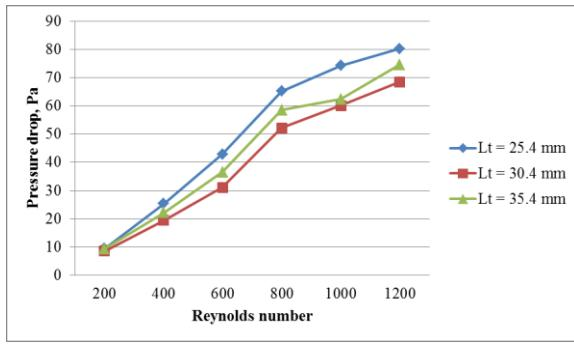
Fig. 11: Effect of varying transverse tube pitch on pressure drop variation for Wavy fin In-line Configuration
