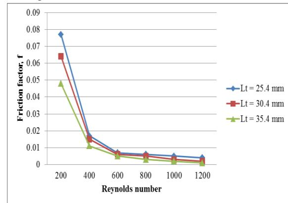
Fig. 14: Effect of varying transverse tube pitch on friction factor variation for Wavy fin In-line Configuration
