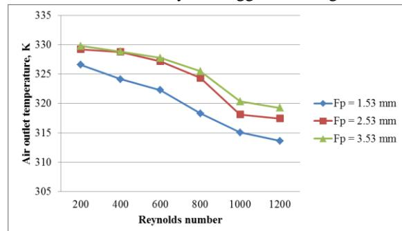
Fig. 35: Effect of varying fin tube pitch on air outlet temperature variation for wavy fin staggered configuration
