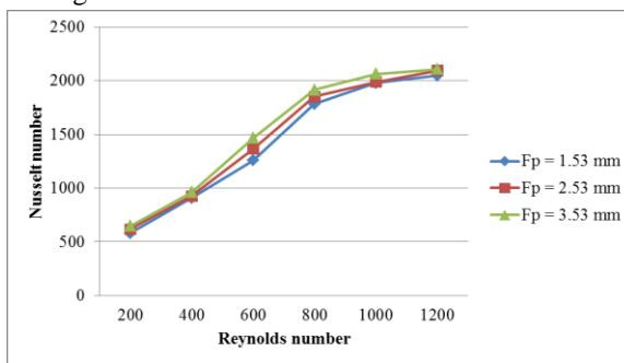
Fig. 19: Effect of varying fin pitch on Nusselt number variation for Wavy fin In-line Configuration
