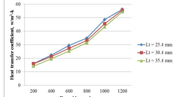
Fig. 31: Effect of varying longitudinal tube pitch on heat transfer coefficient for wavy fin staggered configuration
