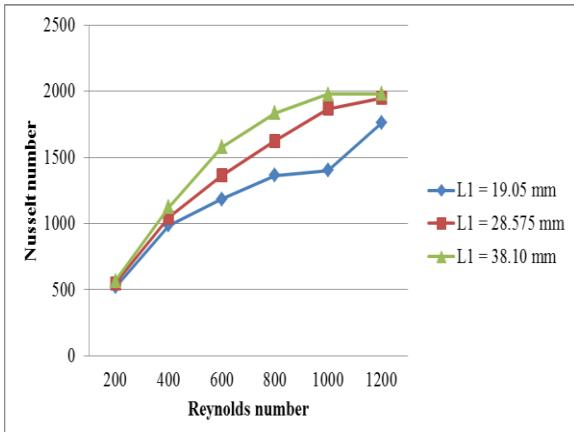
Fig. 7: Effect of varying longitudinal tube pitch on Nusselt number variation for Wavy fin In-line Configuration
