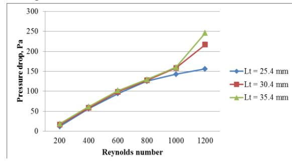
Fig. 30: Effect of varying longitudinal tube pitch on pressure drop for wavy fin staggered configuration
