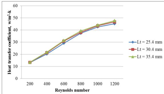
Fig. 12: Effect of varying transverse tube pitch on
