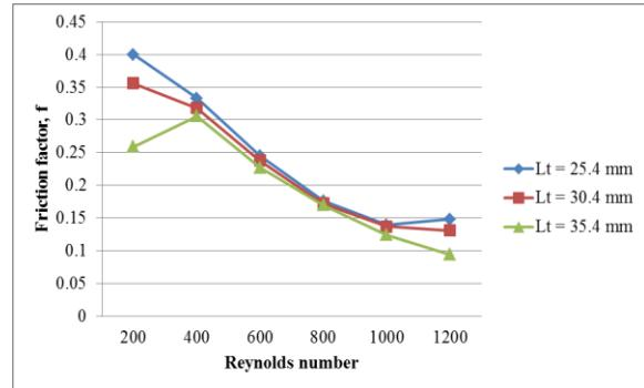
Fig. 33: Effect of varying longitudinal tube pitch on friction factor for wavy fin staggered configuration
