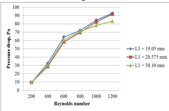
Fig. 5: Effect of varying longitudinal tube pitch on pressure drop variation for Wavy fin In-line Configuration
