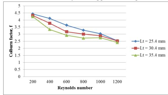
Fig. 34: Effect of varying longitudinal tube pitch on Colburn factor for wavy fin staggered configuration
