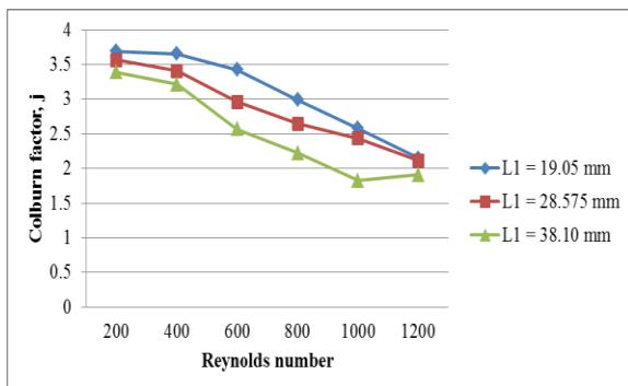
Fig. 9: Effect of varying longitudinal tube pitch on Colburn factor variation for Wavy fin In-line Configuration
