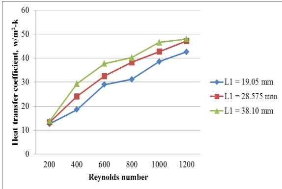
Fig. 6: Effect of varying longitudinal tube pitch on heat transfer coefficient variation for Wavy fin In-line Configuration
