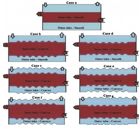
Fig. 1: Different corrugated tubes in a DPHE
