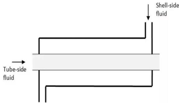
Fig. 3: Double pipe heat exchanger
