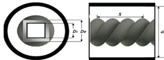
Fig. 2: Twisted inner tube of the DPHE
