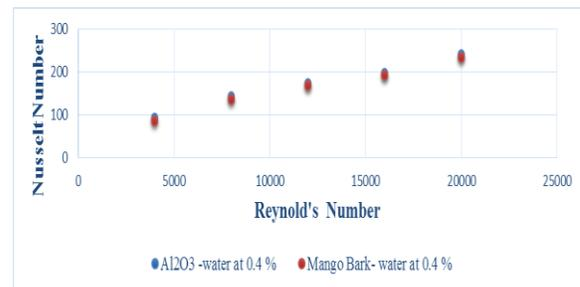
Figure 6 Comparison of Nusselt number for (Al<sub>2</sub>O<sub>3</sub>)-
