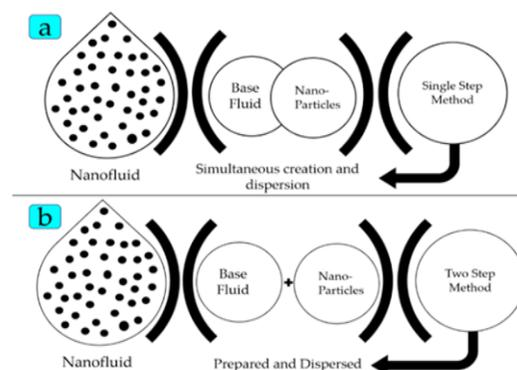
Figure 1: (a) One-step preparation, (b) two-step process of Nano-fluids.
