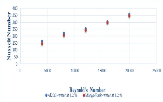
Figure 8. Comparison of Nusselt number for (Al<sub>2</sub>O<sub>3</sub>)-water and Mango bark-water nano fluids at 1.2 % volume fraction
