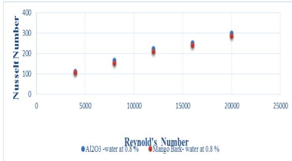
Figure 7. Comparison of Nusselt number for (Al<sub>2</sub>O<sub>3</sub>)-water and Mango bark-water nano fluids at 0.8 % volume fraction
