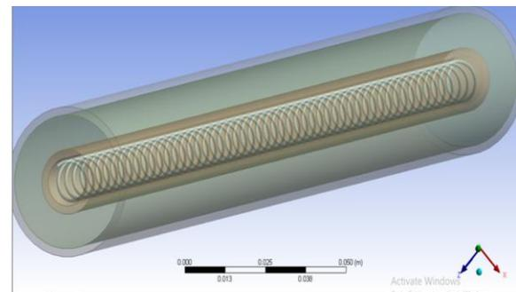
Figure 2. Solid model of heat exchanger with helical turbulator
