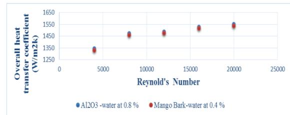
Figure 4. Comparison of overall heat transfer coefficient for (Al<sub>2</sub>O<sub>3</sub>)-water and Mango bark-water nano fluids at 0.8 % volume fraction
