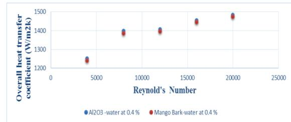
Figure 3. Comparison of overall heat transfer coefficient for (Al<sub>2</sub>O<sub>3</sub>)-water and Mango bark-water nano fluids at 0.4 % volume fraction
