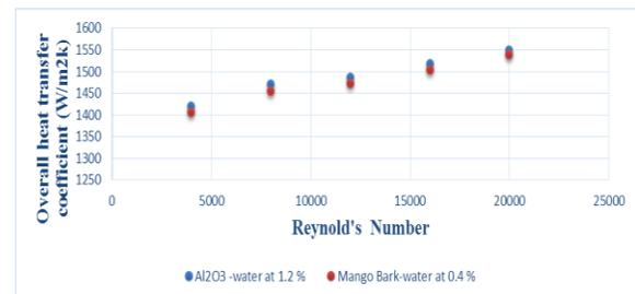
Figure 5. Comparison of overall heat transfer coefficient for (Al<sub>2</sub>O<sub>3</sub>)-water and Mango bark-water nano fluids at 1.2 % volume fraction
