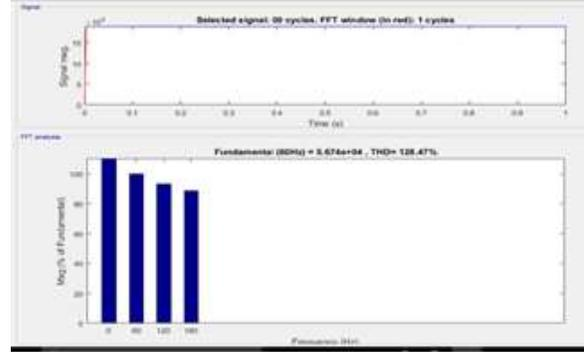
Figure (a):Linear load without STATCOM
