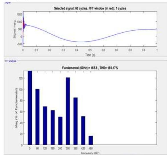
Figure (b): Non-Linear load with STATCOM
