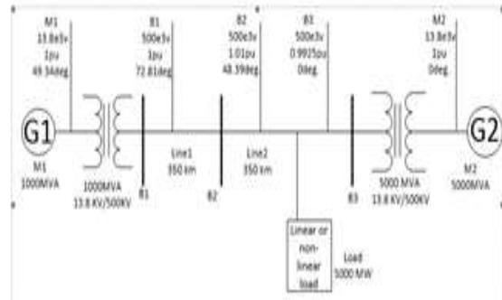
Figure 2: Single line diagram of Two Machine System
