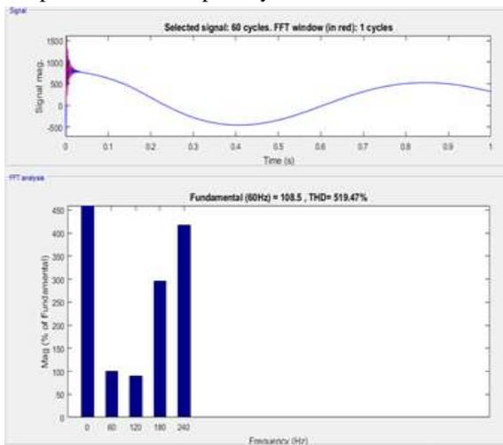
Figure (a): Non-Linear load without STATCOM
