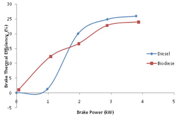
Graph shows variation in brake thermal efficiency for different fuels. Lower brake thermal efficiency is observed with cotton seed bio diesel due to its higher viscosity and low volatility. Due to higher viscosity, injection of larger droplets causes slow evaporation, poor air- fuel mixing and slow combustion which results in lower thermal efficiency.
