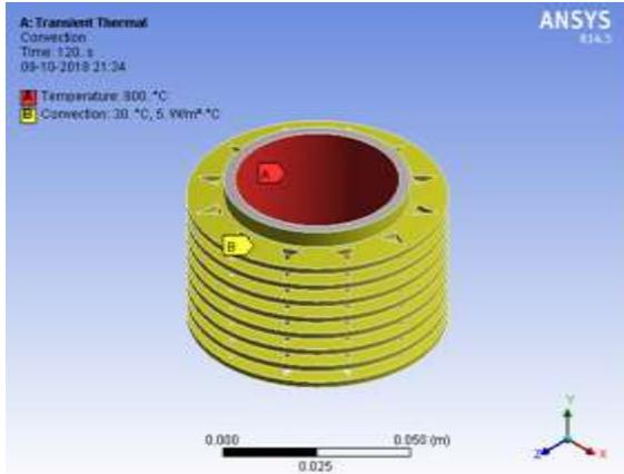
Fig 4 The Named selection of cylindrical block having circular fins with triangular holes.
