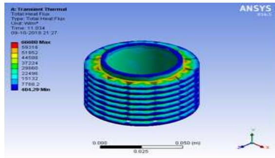
Fig 9 Total Heat flux contour of cylindrical block having Magnesium alloy circular fin with triangular hole
