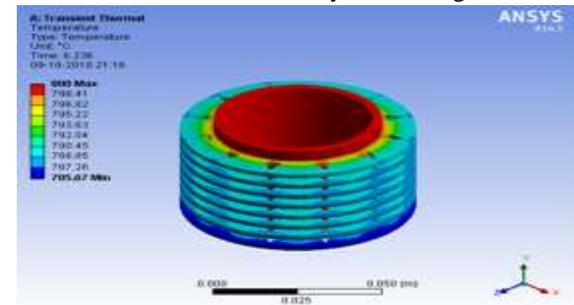
Fig 5 Temperature contour of cylindrical block having Aluminium alloy circular fin with triangular hole
