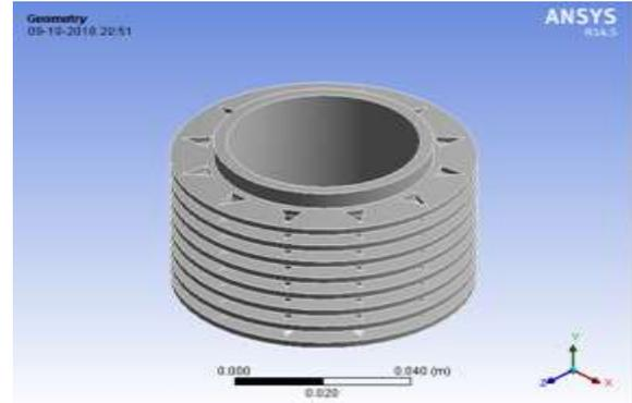
Fig 2 Geometry of cylindrical block having circular fins with triangular holes.
