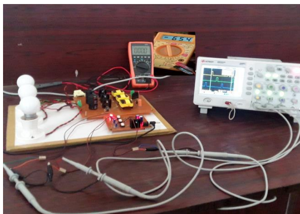
Fig. 14. Experimental setup of a PI control dc-dc interleaved boost converter
