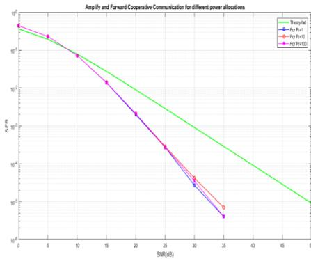
Fig:9 comparison of BER with and without relay when  $P_t = 1, 10, 100$  miliwatt
