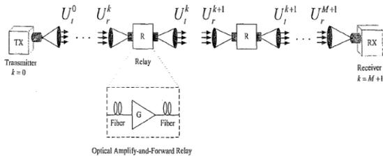
Fig:-1 An All-Optical multihop FSO Communication System
