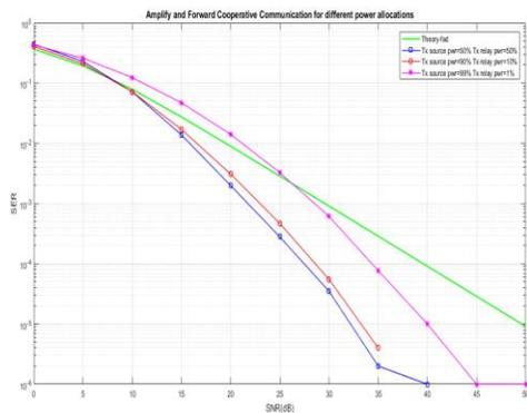
Fig-10 BER if total transmit power distribution for different percentage to source and relay (source have more power compare to relay)
