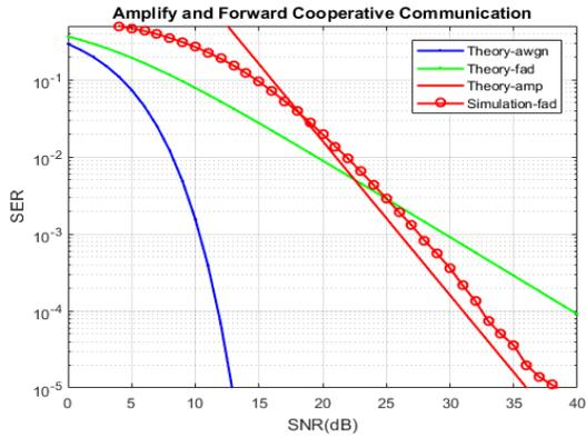
Fig:8 comparison of BER when  $P_t = 100$  mW
