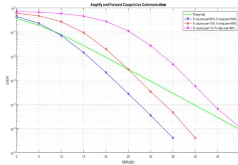
Fig:-11BER if total transmit power distribution for different percentage to source and relay (source have less power compare to relay)
