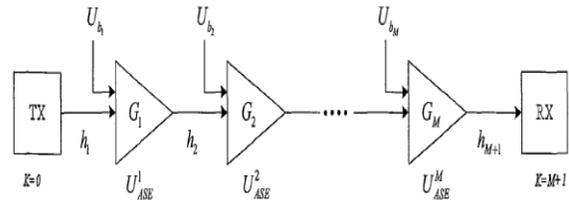
Figure:3 Optical Amplify-and-Forward multihop FSO Systems
