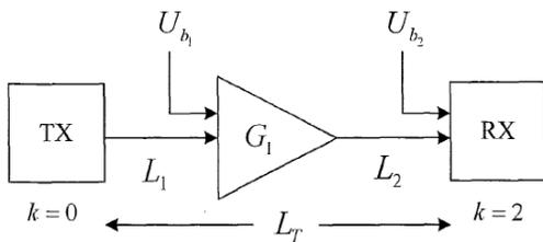
Figure:4 An OAF multihop FSO System with M= 1
