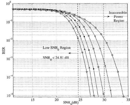
Figure:6 BER versus  $SNR_0$  for a 3 km link and different number of relays  $M$  at  $BR= 10$  Gbps, no fading effect is considered.
