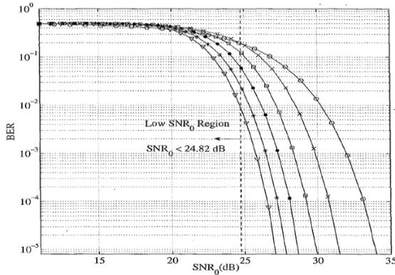
Figure :5 BER versus  $SNR_0$  for a 3 km link and different number of relays  $M$  at  $BR= 1.25$  Gbps, no fading effect is considered.
