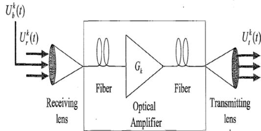
Figure-2 Structure of OAF Relays
