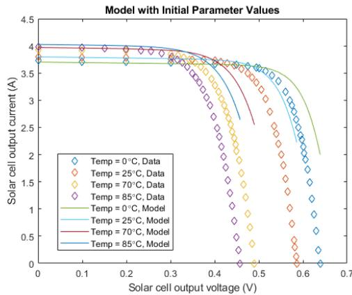
Figure 5 Solar Cell Output
