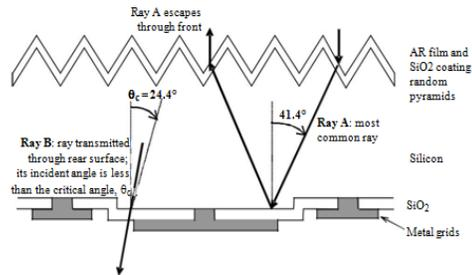
Figure 4 Schematic diagram of A-300 solar cell The rear surface is planar and coated with  $\text{SiO}_2$  except where the metal makes contact to silicon. The metal constitutes the positive and negative electrodes, and it forms a pattern of interdigitated fingers over the most of the cell.
