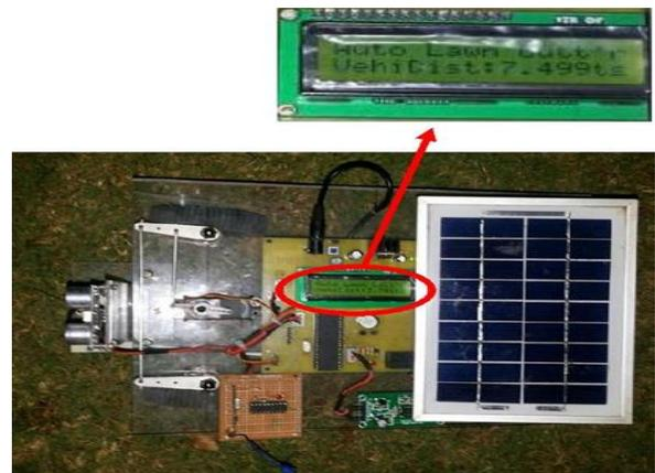
4.3: Displaying measured distance between sensor and obstacle on LCD display
