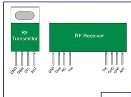
Figure 3.3: RF transmitter and receiver
