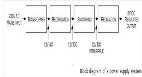
Figure 3.4: Generation of power supply Transformer – steps down high voltage AC mains to low voltage AC. Rectifier- converts AC to DC but the DC output is varying. Smoothing- smoothness the DC from varying greatly to a small ripple. Regulator-eliminates ripple by setting DC output to a fixed voltage
