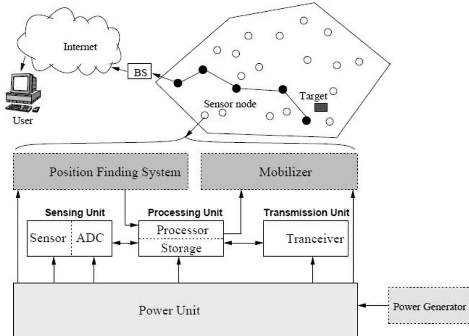
Figure 1. The components of a sensor node
