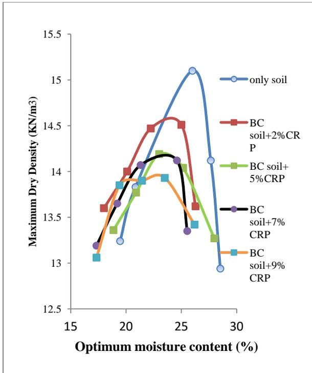
Figure.5 Compaction curves for BC soil with varying percentage of CRP
