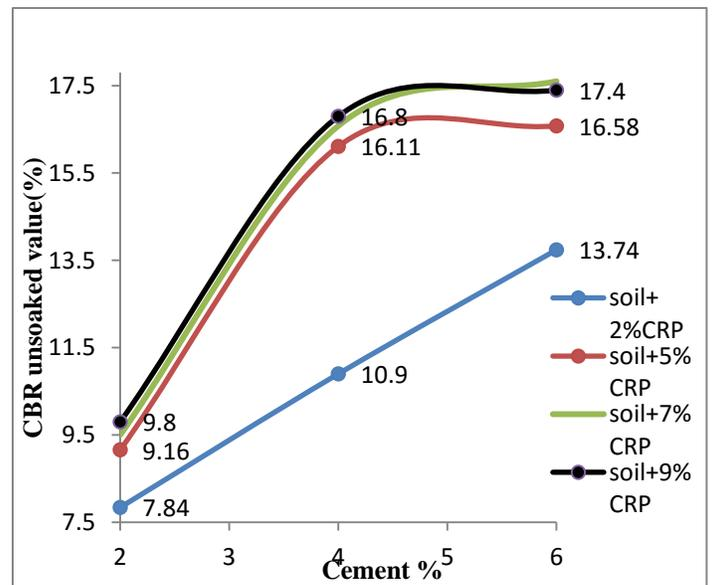
Figure.8 Variation of CBR of BC soil-CRP mix with varying percentage of cement
