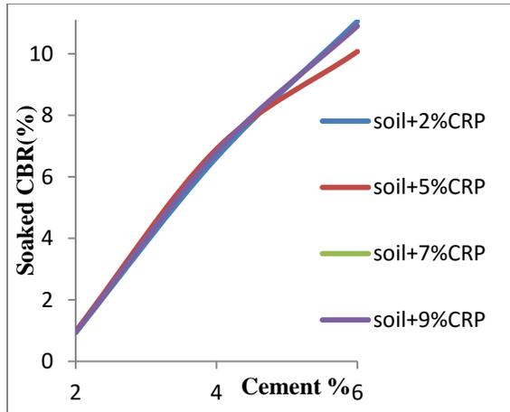
Figure.9 Variation of CBR of BC soil-CRP mix with varying percentage of cement
