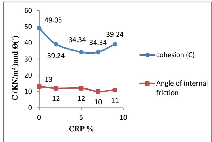
Figure.7 Variation of cohesion and angle of internal friction with CRP %
