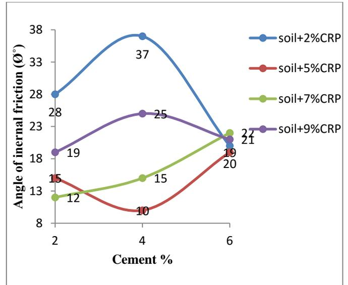
Figure.11 Variation of Angle of internal friction of BC soil-CRP mix with varying cement %
