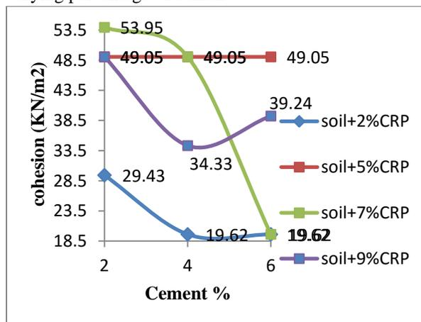
Figure.10 Variation of cohesion of BC soil-CRP mix with Cement %
