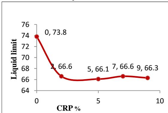
Fig.2 Variation of Liquid limit with CRP content
