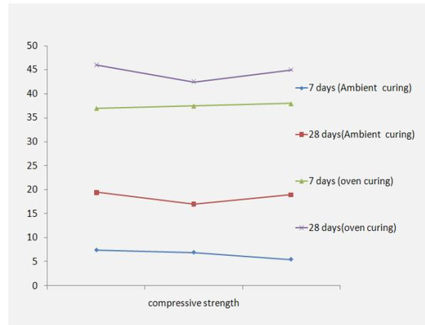
Fig.1. Graphical Representation of Compressive Strength of Geopolymer Concrete
