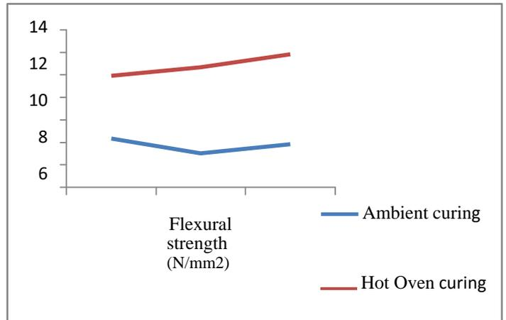
**Fig.3.Graphical Representation of Flexural Strength of Geopolymer Concrete**
