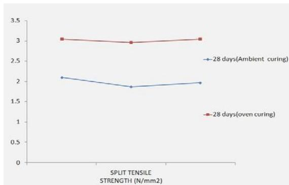
**Fig.2.Graphical Representation of split tensile Strength of Geopolymer Concrete**
