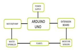
This project uses Arduino Uno to controls the motor. Follow the schematic to connect the Arduino to the motor driver, and the driver to the water pump. The motor can be driven by a 9 volt battery, and current measurements show us that battery life. The Arduino
