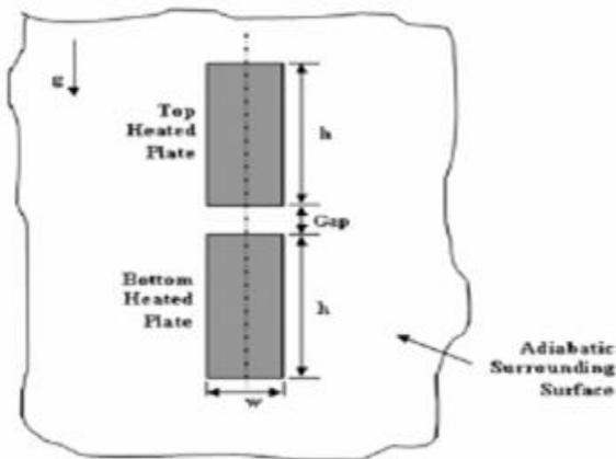
Fig. 2: Vertically adjacent plate flow situation considered. The present work arises from the fact that when there are two adjacent narrow flat plates with a relatively small gap between the plates the flow near the adjacent plates alters the nature of the flow compared to that over a single narrow plate and this can lead to a significant change in the mean heat transfer rate compared to that from a single isolated plate under the same conditions as shown in Fig.2.
