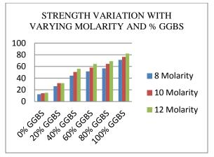
The addition of GGBS to replace fly ash increases the compressive strength progressively. But it accelerates the initial setting time to less than 6 minutes when it completely replaces the fly ash content in geopolymer concrete. Hence it is observed that the GGBS content content in GPC can well be optimized based on the setting time.
