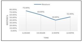
(c) illustrates the humidity reading of the garden at different time slots. Time is taken on the x-axis, while the humidity values are taken on the y-axis. The difference in recording the humidity is 4 hours in Fig. (c). Initially, the humidity value is high in the morning, but with sunrise, it decreases.
