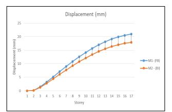
Graph 2 Time History - Displacement (mm) From the above table & graph, we can observe that percentage variation for Displacement for Time History Analysis for model 2 is less than model 1. The variation is found to be 15-20% less for model having Base Isolation than model have fix base only.
