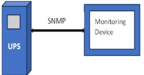
Figure 1: Data exchange between UPS and Monitoring Device using SNMP Protocol
