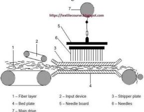
FIG NEEDLE PUNCHING PROCESS
