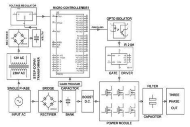
Fig. Variable Frequency Drive
