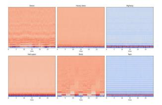
B. Mel Spectrogram: A visual representation of the spectrum of frequencies of a sound signal as it varies with time. Spectrograms help in identifying time-varying frequency components, distinguishing drones from other environmental sounds.
