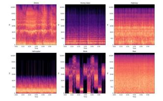
c. Frequency Domain Features: Further analyzing the frequency content of the sound, features like Spectral Centroid and Spectral Bandwidth provide insights into the spectral distribution and bandwidth of the signal.
