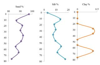
Fig. 2. Down-core variation of sand, silt and clay in river core sample
