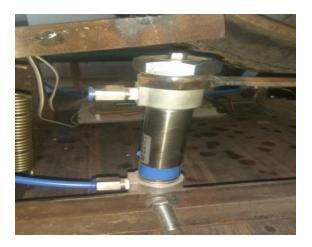
*C. Solenoid Valve* :A solenoid valve is an electromechanically operated valve. The valve is controlled by an electric current through a solenoid: in the case of a two-port valve the flow is switched on or off. The compressed air from the reservoir flows through the solenoid valve as soon as it receives signal from the microcontroller unit and the piston-cylinder arrangement operates to engage the secondary lever to the primary one.
