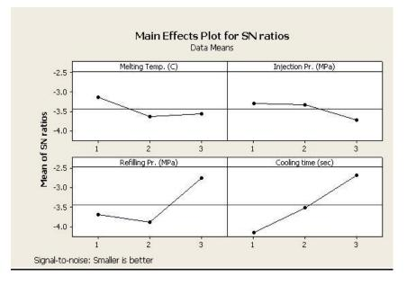
Optimization of Injection Moulding Process Parameters in the Moulding of Low...
