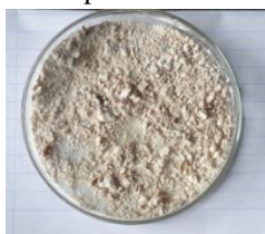
Figure VII: Precipitate formed by incorporating of oven dried precipitate and anti-caking agent (corn starch)
