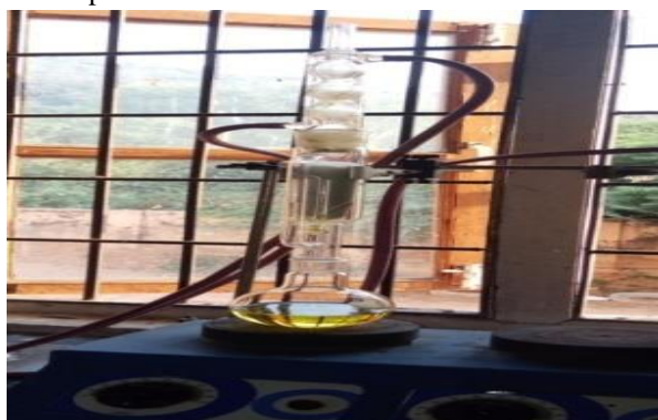
Figure 1: Solvent Extraction Process (Soxhlet Apparatus)
