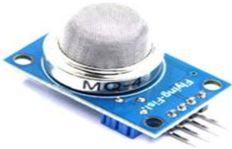
Fig. 4. MQ4 Methane Gas Sensor
