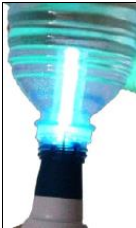
Fig. 2. Use of UV light for water purification.
