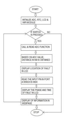
Flow Chart of Fault Detection System
