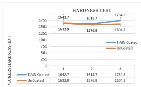
Figure 6 Line Graph for the Vickers Hardness Test (HV)
