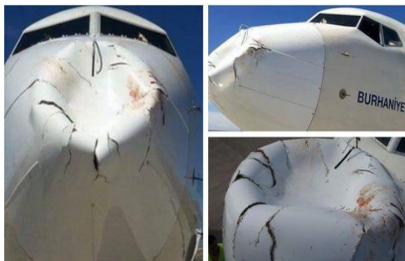
Fig.2. Result of bird strike on Radome
