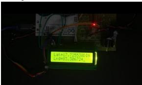
Fig 10: location tracing display
