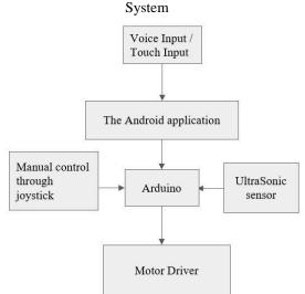
Fig 4.3: Overall functioning with respect to Arduino UNO
