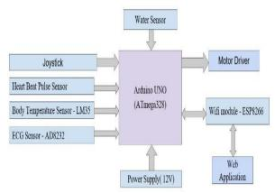
Fig 4.1: Overall functioning with respect to Arduino UNO
