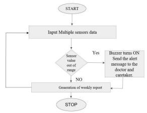
Fig 4.2: Block diagram for Health-Monitoring
