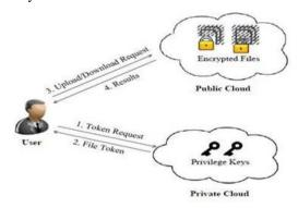
Figure 1: Architecture for Authorized Deduplication This work known a company by where the employee data such as name, password, email id, contact number and designation is registered by admin or owner of the company based on his userid and password employees of the company able to perform operations such as file upload download and duplicate checks on the files based on his privileges.
