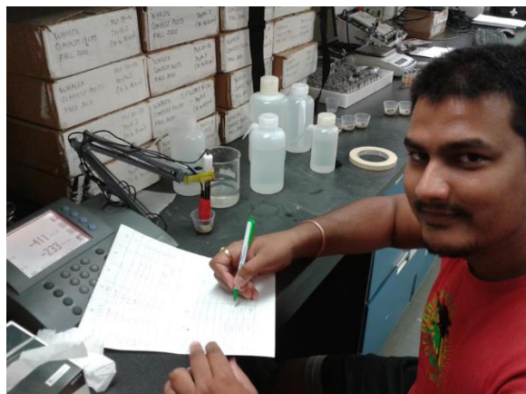
Figure 1: Real-time soil phosphate ion measurement setup
