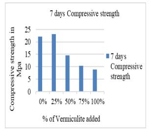
Fig 6.2 Variation of 7 days compressive strength Variation of 28 Days Compressive Strength:
