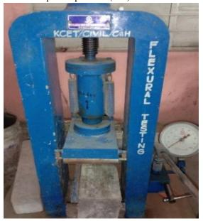
Fig 6.4 Experimental setup for flexural strength test Table 6.2 Flexural strength of beam
