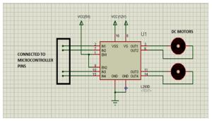
fig 5. Motor Interfacing
