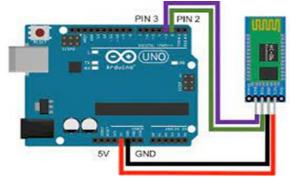
fig 6. Bluetooth Interfacing
