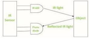
types of radiations are invisible to our eyes, but the infrared sensor can detect these radiations. When IR light falls on the photodiode, the resistances and the output voltages will change in proportion to the magnitude of the IR light received [5][6].
