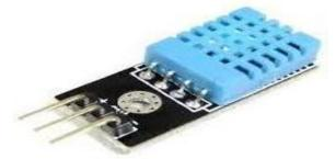
The humidity sensing device DHT11 is a moisture holding substrate with the electrodes applied to the surface. The change in resistance between the two electrodes is proportional to the relative humidity. Humidity sensors work by detecting changes that alter electrical currents or temperature in the air.[2]
