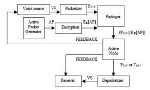
Figure 1: Architectural block diagram
