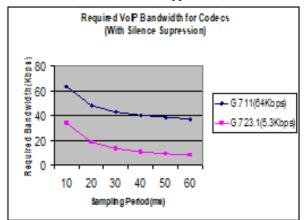
Figure 3: Required VoIP bandwidth for Codecs (With Silence Suppression)
