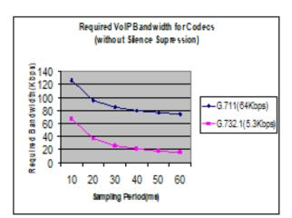
Figure 2: Required VoIP bandwidth for Codecs (Without silence suppression)
