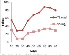
Fig. 3: Variation of TS & VS for Sewage sludge as Inoculum
